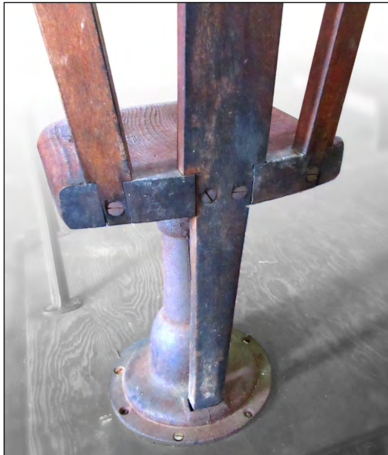
Fig. 1.12 Detail of joinery showing the prominent screw heads. (© Philip Carlino, all rights reserved.)
