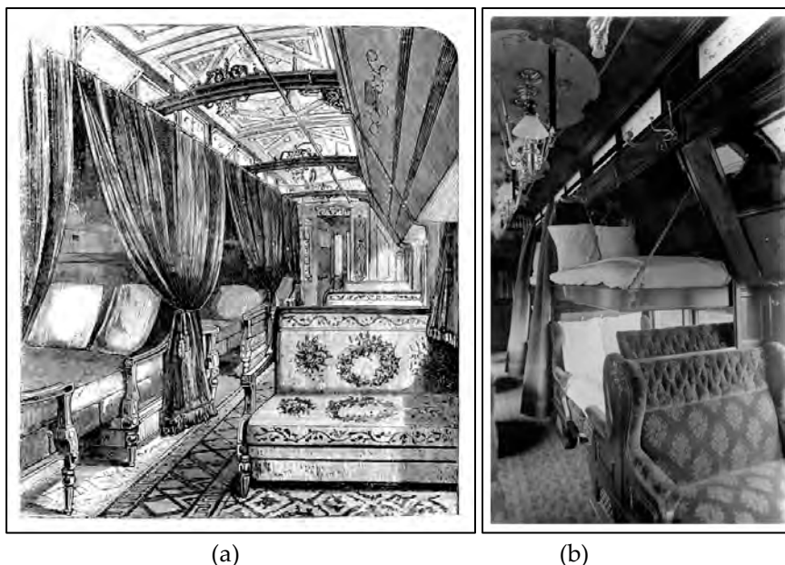
Fig. 4.19 a. An 1869 engraving of one of the first Pullman sleeping cars; and b. a photograph circa 1890 of the Pullman sleeping car “Anton” showing the basic form remained the same throughout the nineteenth century. In the photograph the partition at the foot of the berth has yet to be bolted in place, by the porter and the rod for the curtains appears at center. (a London Illustrated News , October 2, 1869, 336; b. Pullman Palace Car Company Photographs, Archives Center, National Museum of American History, Smithsonian Institution, Pullman negative 2827.)
